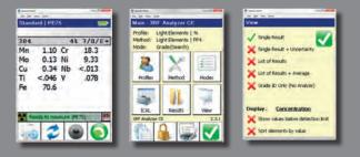
The software delivered with the SPECTRO xSORT enables not only display of the measurement screen on the PC monitor. It also makes it possible, for example, to enter sample identification, to delete measurement values, or to open the menu so that changes in the instrument settings can be made.
