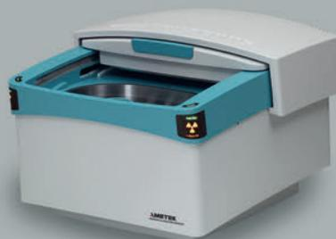
targeted matrices. An innovative 50 W / 60 kV X-ray tube and unique new adaptive excitation technology furnish the highest possible sensitivity, optimized to target elements
