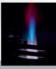
In plasma viewing, "dual" usually denotes both radial and axial views. Example: to increase sensitivity, some newer vertical-torch dual-view instruments complement their radial view via a second periscope coupled axial view interface above the plasma. However, this adds significant light loss, interferences, contamination, and thermal stressing of interface components.
