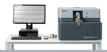
Both versions feature a temperature-stabilized system, heating both optics and requiring no external cooling. Both versions are available as floor-mounted units with optional PC stand, or benchtop models.
