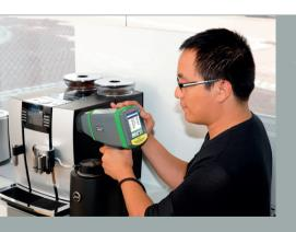
THIS HANDHELD ENERGY DISPERSIVE X-RAY FLUORESCENCE (EDXRF) SPECTROMETER has exceptional performance for this class of instrument, and can provide laboratory quality screening results in a matter of seconds. The SPECTRO xSORT has been optimized for fatigue-free on-site measurements.
